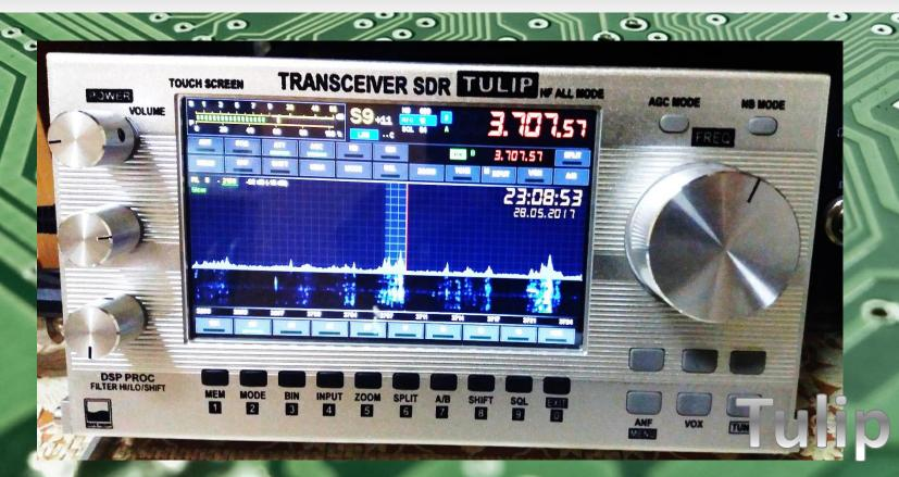
The kit obtained from Artur SP3OSJ contains housing, buttons encoders and volume control screens of modules supports tilt wiring (excellently performed) jacks for headphone, microphone in / out audio socket battery bios, controls button caps and end caps.
