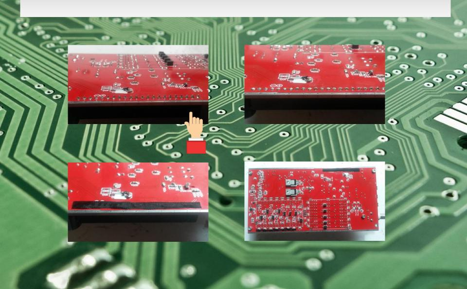
Mounting components must be done very carefully. In the first stage we mounted all resistors, inductors, capacitors and all stabilizers. At this stage we made the first hot checks, checking the main stresses in the diagram. In the second phase we Tufted Switching Power 5V, all the relays and connectors. Then at a time starting with PCB3, at the end PCB1 and PCB2 have mounted active components
